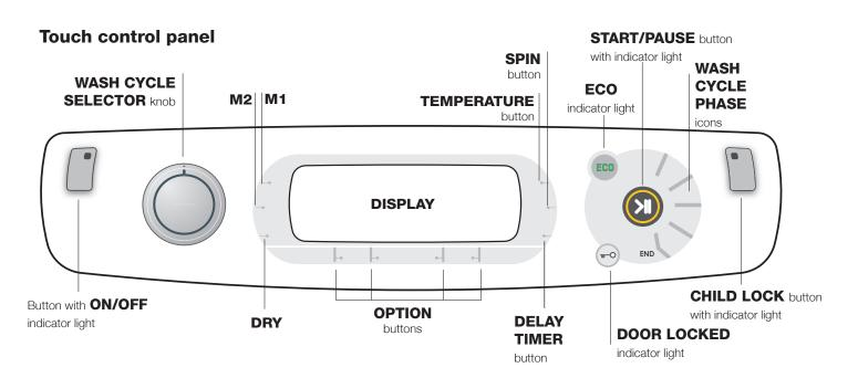
Button with () **ON/OFF** indicator light: press this briefly to switch the machine on or off. The green indicator light indicates that the machine is switched on. To switch off the washer-dryer during the wash cycle, press and hold the button for approximately 3 seconds; if the button is pressed briefly or accidentally the machine will not switch off. If the machine is switched off during a wash cycle, this wash cycle will be cancelled.
